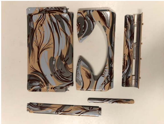
19xx Groma Kolibri with its body plates removed. The metallic beige paint was scraped in several locations and missing.
