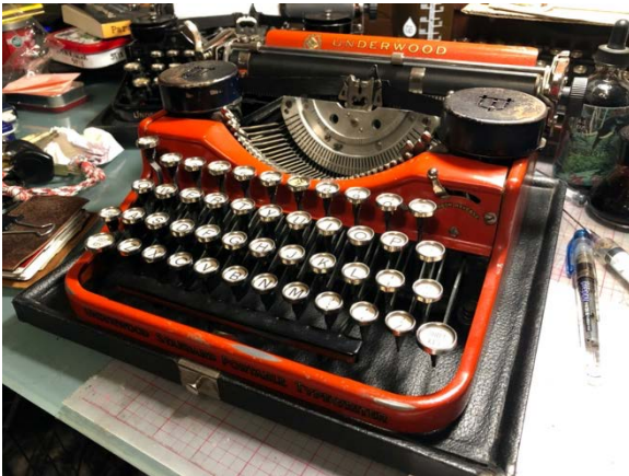
1930 Scarlet Red Underwood 4-Bank This was found in a cardboard box. After I put it back together and tuned it up it worked super – but, was missing the spool covers. I found original spool covers in black. I custom mixed 1-Shot epoxy paint to match the machine.
