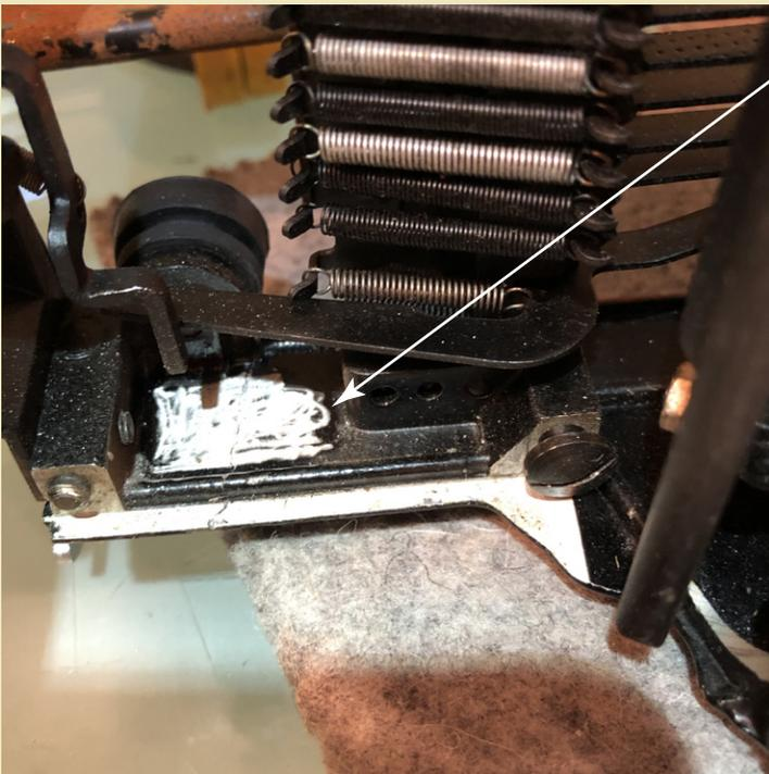
A Dremmel Tool was used to remove the paint so that the weld would have a place to “bite” into. I wanted to get down to the metal instead of gluing to the paint.
