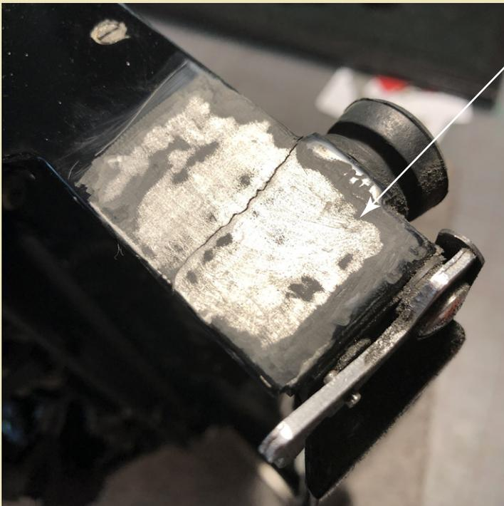
The clamp was removed and the outside paint was removed to the metal with a Dremmel Tool in order for the adhesive to bind directly to the frame.
