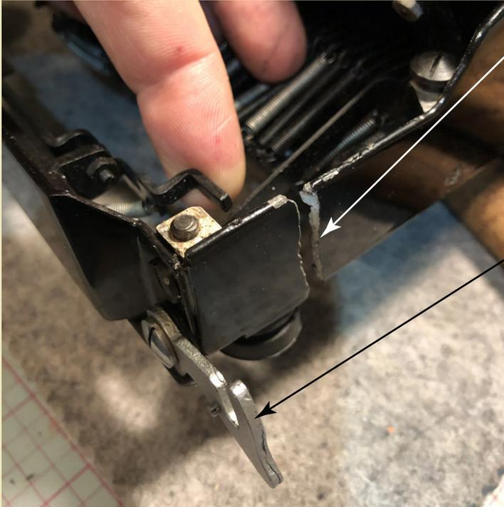
The break was relatively clean and the frame was not bent. The aluminum frame in this area is thin and it makes sense that it would have broken here.
